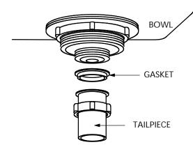
10. Check to be sure the bowl is level side-toside, then tighten the four bolts holding the upper bracket. Level the bowl front-to-back by either raising or lowering the "L" shaped bracket and tighten the single bolt. Connect the fixture to the hot and cold supply lines. Install the trap and connect the drain. Apply a bead of silicone to the back edge of the bowl to seal it to the wall.
