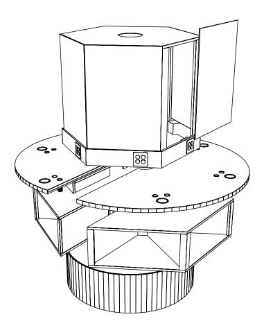
Adjacent cabinets and components should be assembled by fastening through the interior panels with the screws or bolts provided. Tighten securely.
