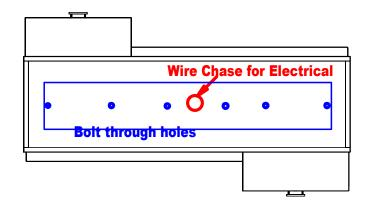
Set soffit on top of assembled station after installing the mirrors. Center the soffit front to-back as well as side-to-side. Attach using provided bolts in the marked holes from the top down.
