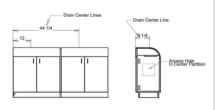
Bolt the left and right cabinets to center cabinet with (4) 1 1/4" beauty bolts. Bolt through interior side panels.
