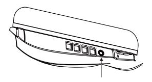
Long press the "safe-lock button" for about two seconds, lighting up the green light around the button, all the keys except the safe-lock button can not be operated. Long press the safe-lock button again for about two seconds, and the green button lights go out, all the keys return to normal operation status.
