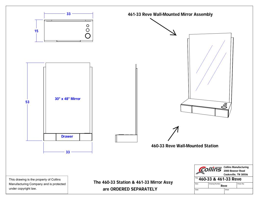
This item is attached to the wall with wood screws. 3" wood screws and decorative washers are provided for wood framed walls. Fasteners for other wall types are to be obtained locally. Screw through the back panel in locations which will be inconspicuous after installation. Suggested locations include: under shelves, behind drawers, and locations hidden by products or supplies.
