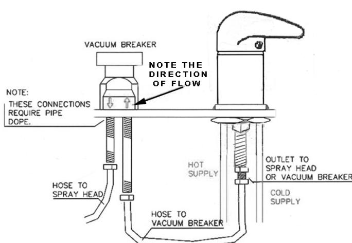
ENGLISH: Arrows on the vacuum breaker indicate directional flow of water. Device will leak and not work properly if installed with water flow reversed.
