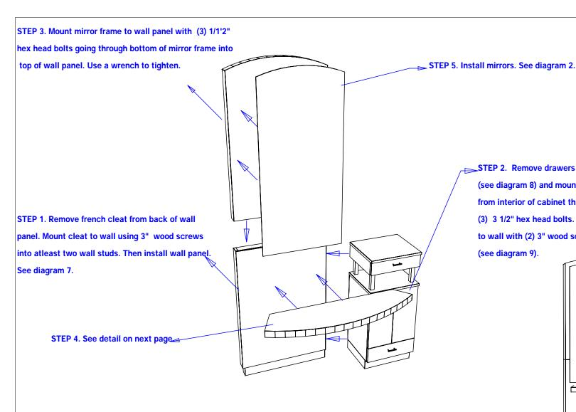
STEP 2. Remove drawers from base cabinet (see diagram 8) and mount it to the wall panel from interior of cabinet through sides with (3) 3 1/2" hex head bolts. Then mount cabinet to wall with (2) 3" wood screws into wall stud (see diagram 9).
