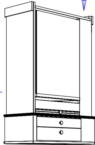
STEP 1. Mount base with legs to wall using (4) 3" wood screws into two wall studs.
