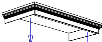
STEP 3. Mount crown cap on top of cabinet by screwing (4) 1 1/2" wood screws through top of crown down into cabinet. See detail below.
