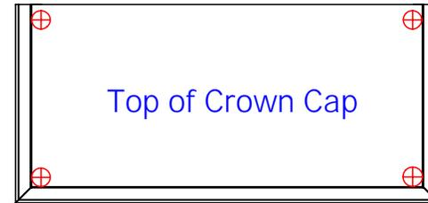
STEP 2. Mount cabinet to base by screwing (4) 1 1/4 wood screws up through the base cleats into the cabinet cleats. Then mount cabinet to wall using (4) 3" wood screws with beauty washers through interior of cabinet at each corner into wall studs.
