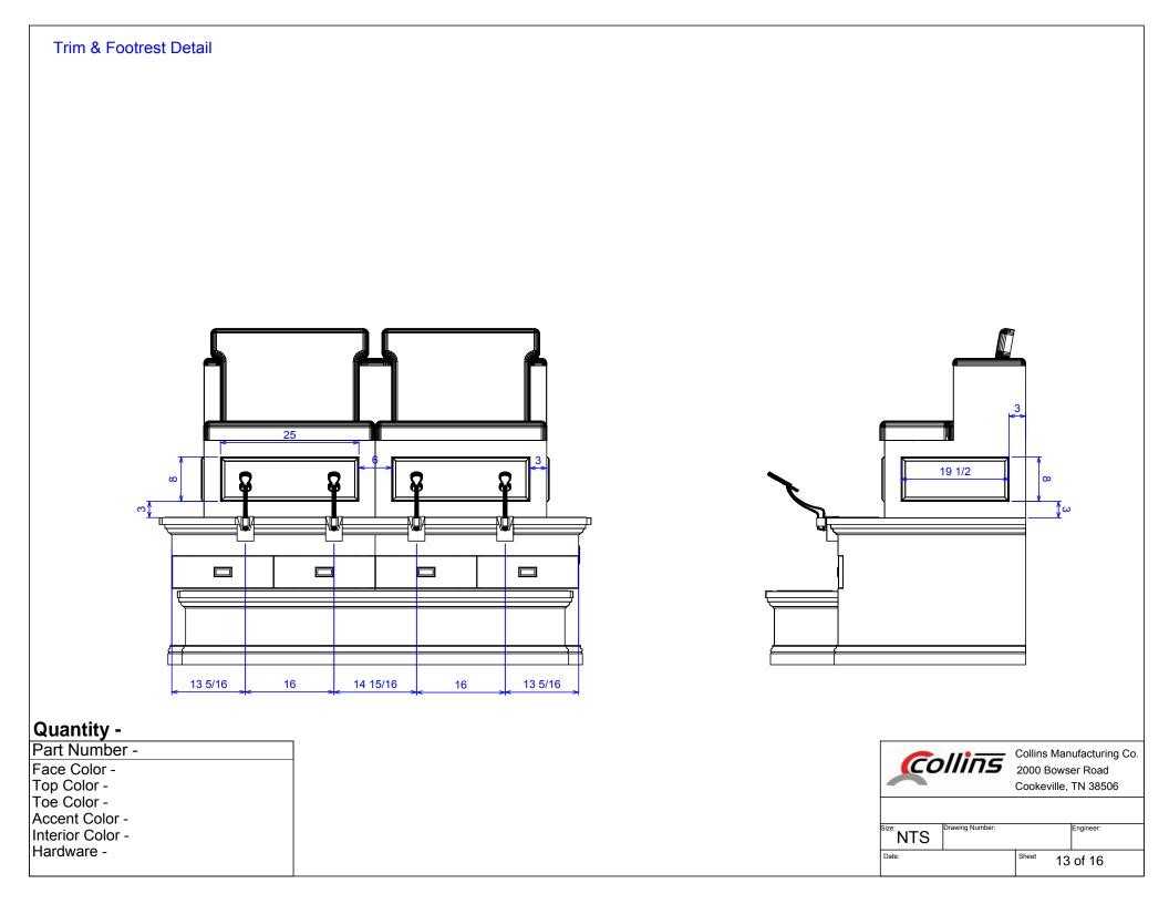
Remove Drawers to access inside of Base Cabinets. The Left and Right Base Cabinets will bolt together with supplied connector bolts.
