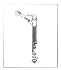
STEP A. Single hole installation Insert all flexible hoses through hole in sink ledge.
