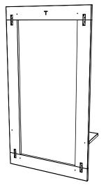
When attaching mirror frame to wall make sure to stay within the inside 2" with screws. The outer 2" will be visable. Note: top frame is marked with a "T".
