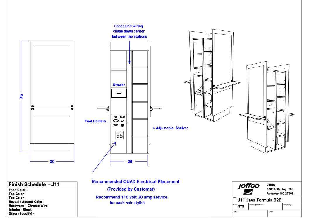
This item is attached to the wall with wood screws. 3" wood screws and decorative washers are provided for wood framed walls. Fasteners for other wall types are to be obtained locally. Screw through the back panel in locations which will be inconspicuous after installation. Suggested locations include: under shelves, behind drawers, and locations hidden by products or supplies.
