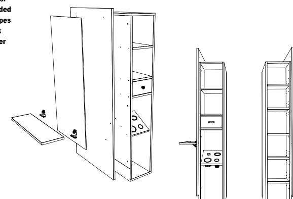
Use the six provided connector bolts and nuts to attach both sides together. Assembly holes are factory drilled.
