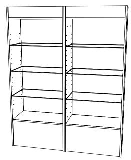
Two unit run...Two center connector legs attached to base and top with bolts and threaded inserts.
