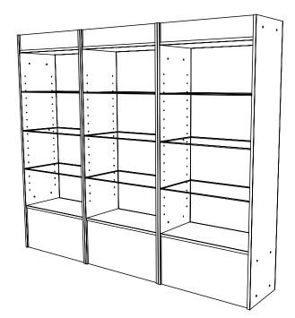
Four unit run...Six center connector legs attached to base and top with bolts and threaded inserts.
