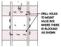
The back plate must also have holes drilled for mounting the Valve Assembly to the wall. Determine the appropriate location for the mounting holes and drill holes in the back plate. Attach the Valve Assembly to the wall.
