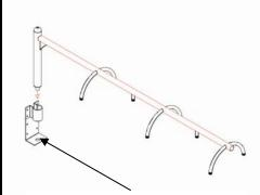
Insert large plastic washer between bottom of Rainbar and bottom of mounting bracket
