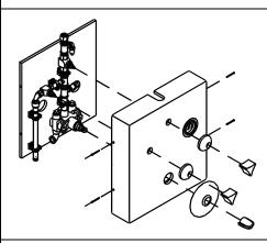
Remove the four screws that connect the cover of the Valve Assembly to the back plate, and remove the cover. The valve handles and their escutcheon must be removed prior to removing the cover. See separate picture illustration for instructions to remove control valve knobs and temperature control valve, and release the escutcheon.
