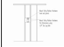
Position the stainless steel mounting bracket on the surface it is to be attached to, according to the diagram, and mark mounting holes. The flange with the large hole is the bottom of the bracket and goes towards the floor.
