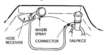
If your bowl is equipped with a vacuum breaker, connect one end of the fixture hose to the inlet side of the vacuum breaker. Connect the other end to the fixture tailpiece. Attach the WhizRSpray hose connector to the vacuum breaker outlet.
