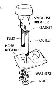
**NOTE:** Install the vacuum breaker as shown. If the vacuum breaker is installed backwards, it will interfere with the Whiz Spray.
