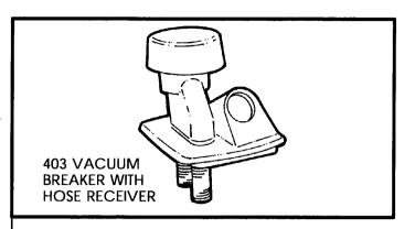
3. Remove the two (2) hex-nuts and washers from the vacuum breaker pipes. Place the vacuum breaker pipes through the holes in the hose receiver as shown. Secure the vacuum breaker to the hose receiver with the washers and hex-nuts.
