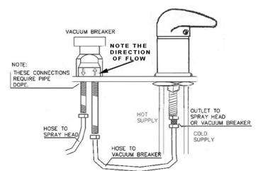
ENGLISH: Arrows on the vacuum breaker indicate directional flow of water. Device will leak and not work properly if installed with water flow reversed.
