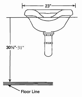
The depicted mounting height is the recommended mounting height for bowls of this design when used hydraulic all-purpose chairs.
